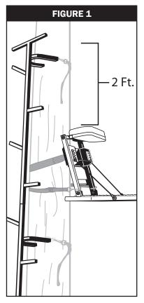
WARNING! Your climbing system was designed for installation on trees with a minimum diameter of nine (9) inches (23 cm) and a maximum diameter of (20) inches (51 cm). DO NOT use your Big Game® product(s) on trees with trunk diameters that do not meet this minimum/maximum diameter requirement. Failure to follow these instructions may result in serious injury or death!
